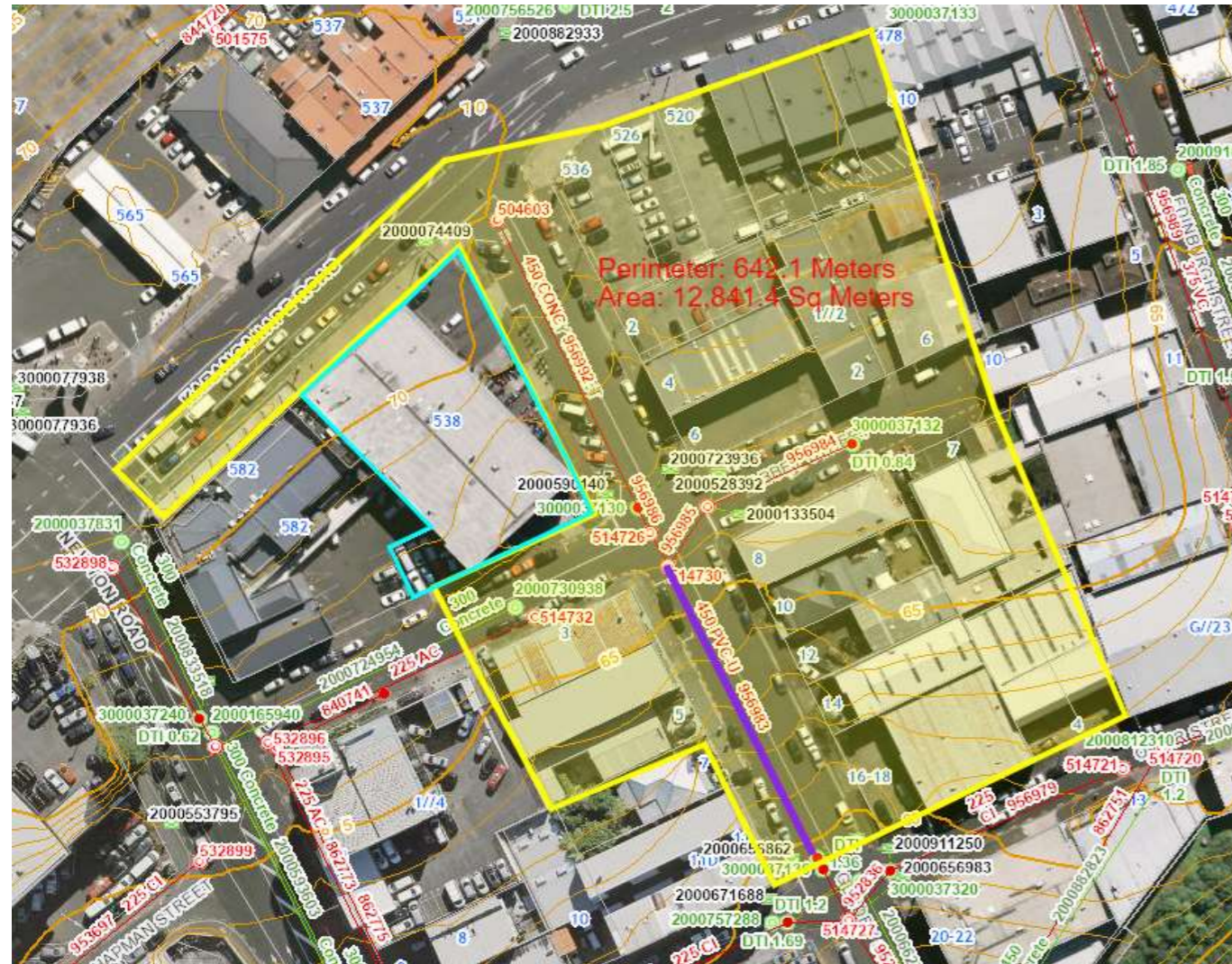
Stormwater Catchment - Assumed All impervious 12850 m2
