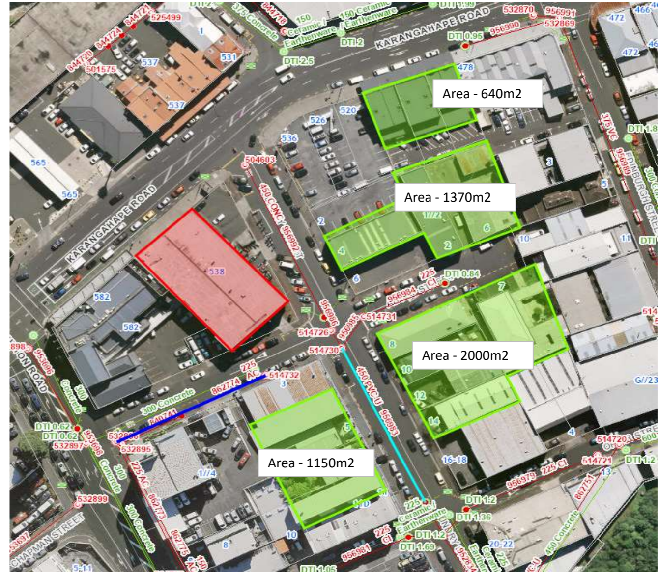
Wastewater Catchment - Assumed 5160 m2 is 2 storey (total 10320 m2) and 80% of total is occupied with offices.
